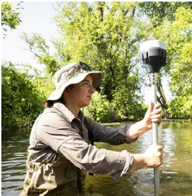
Figure 4.3. GNSS receiver was used to calculate location and sediment depth. Photo by Bryce Richter/UW-Madison
