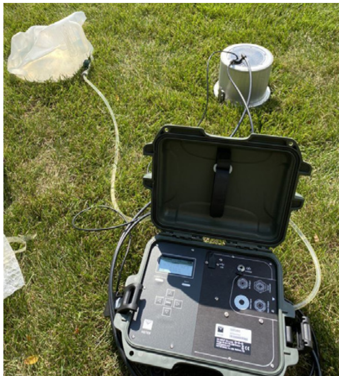
Winkelman and his WRM group conducted infiltrometer testing to determine the infiltration rate of water into the soil.
