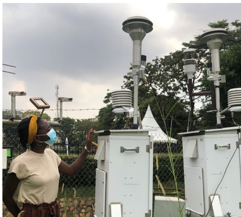
Lsoto views two air quality reference monitors owned by AirQo located at Makerere University weather station. The two reference monitors bring the total number of reference monitors to three in the country including the first one owned by and housed at the US embassy. The two reference monitors are used to calibrate the low-cost air quality monitors. Photo credit: Dorothy Lsoto
