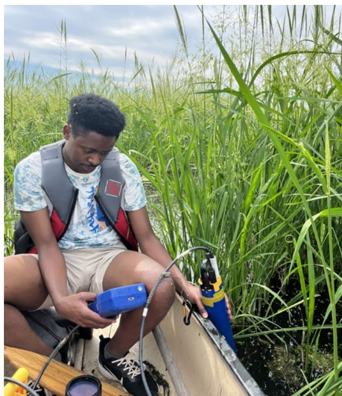
Cohort member Daniel Igirimbabazi collects water chemistry data via YSI Sonde. Photo courtesy of Hannah Stuart
