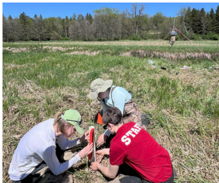
WRM students Katie Hietpas, Hanna Kollbaum, and Alayne Kulp work to install a shallow well to monitor groundwater flow in the wetland surrounding Fancy Creek. Photo by Sophie Van Alsbury
