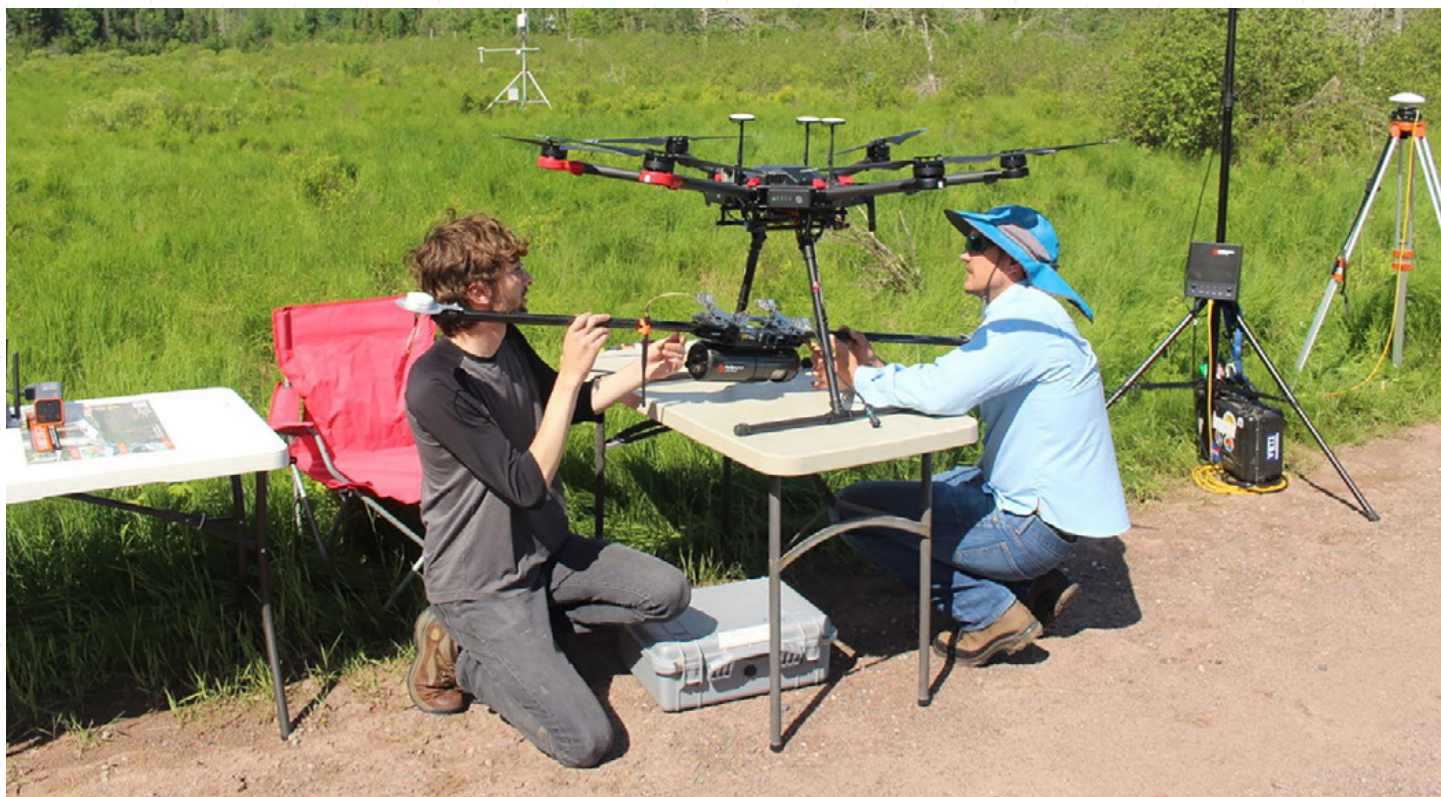
Christian Andresen (left) prepares a LIDAR-equipped drone for remote sensing. Photo courtesy of Christian Andersen (3)
