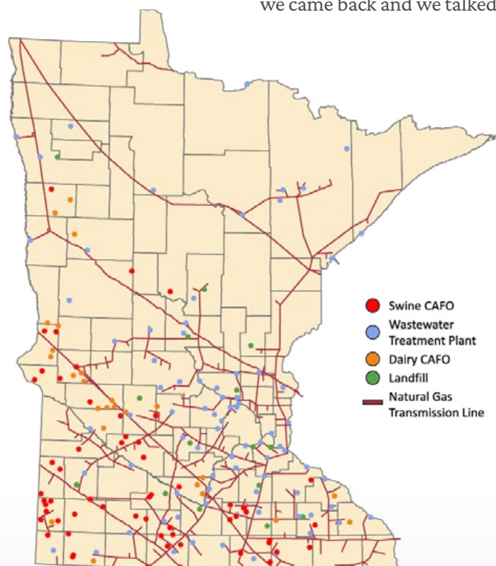
Locations of viable RNG sources relative to existing natural gas transmission pipelines in MN. The existing pipeline infrastructure is shown as dark red lines.
